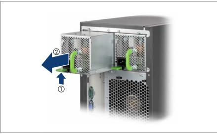
Figure 20: Unlocking and removing the power supply unit
